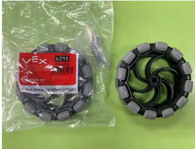
圖 7.萬向輪(Omni-directional wheels)
